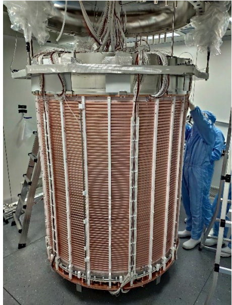
Figure 4 Time Projection Chamber (TPC) of the XENONnT detector for dark matter particles, utilizing liquid xenon as detection medium. Picture taken from https://xenon-experiment.org/
