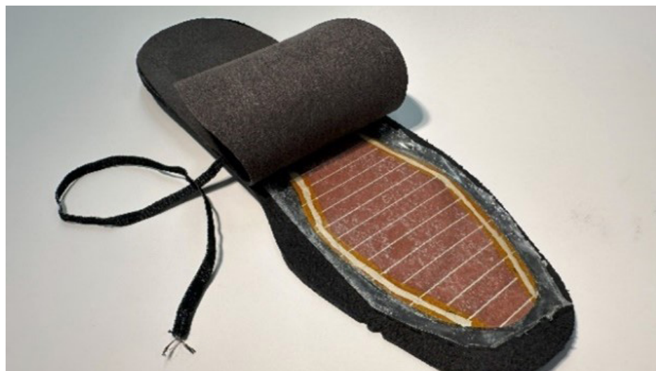
The first prototype of a heated shoe sole including qCella's heating mat
